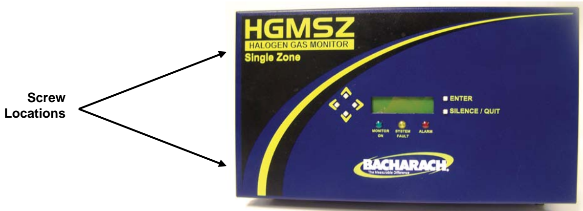
Figure 1. Screw Locations on Single Zone Chassis
