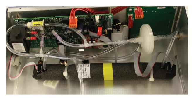
Figure 2. Internal Components Showing the IR Sensor (Bench) of a PGM-IR
