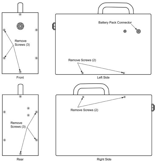
Figure 3. Disassembling the Chassis
