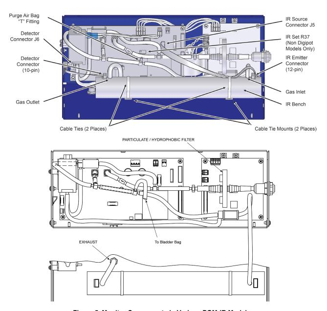
Figure 5. Monitor Components in Various PGM-IR Models
