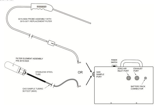
Connecting the Gas Sample Line or Probe
