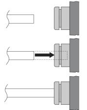
To connect the elbow connector to the zero air filter PTC fitting, firmly push the elbow into the hole in the center of the connector until it seats in the connector. Refer to the figures at the left.
