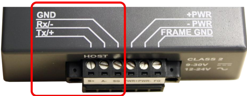
Figure 6. RS-485 Network Connections (Baud Always = 19200)
