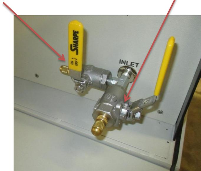
The inlet valve plumbing to the source container must be leak tested before operating the machine to guard against Agent loss. Leaks in the inlet connections will also allow ambient air to enter the machine during the vapor recovery cycle.
