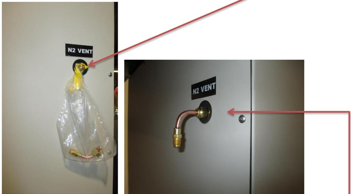
Connect the Deflector Tube to the Vent Port finger tight. Then just lightly tighten snug with a 5/8" open end wrench. Do not over tighten: this may twist the internal plumbing of the machine.
