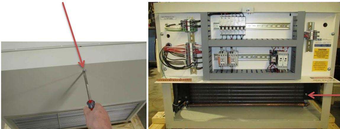
The condenser coil is directly below the main wire box of the machine.
