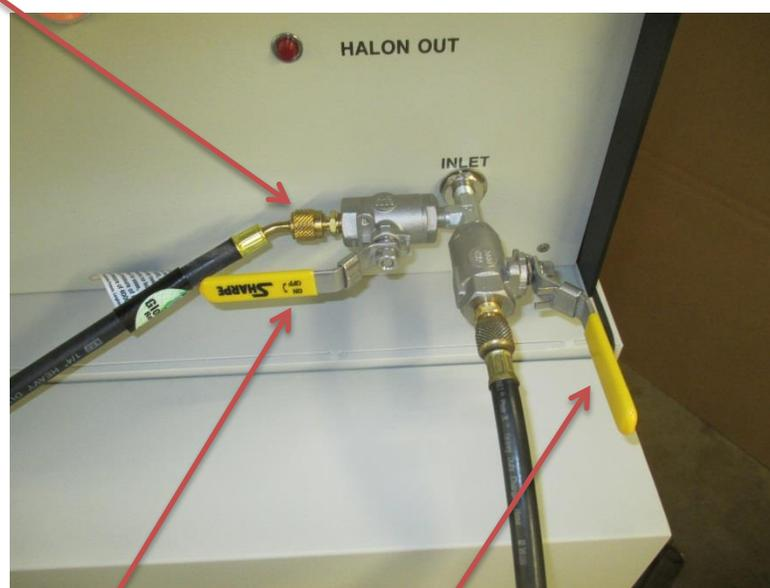
3. Open the Evacuation Valve and the Manual Inlet Valve to pressurize the plumbing with the nitrogen and leak test the plumbing connections using leak detect fluid.
