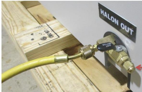
14. Open the vapor valve of the storage container if it is closed.
