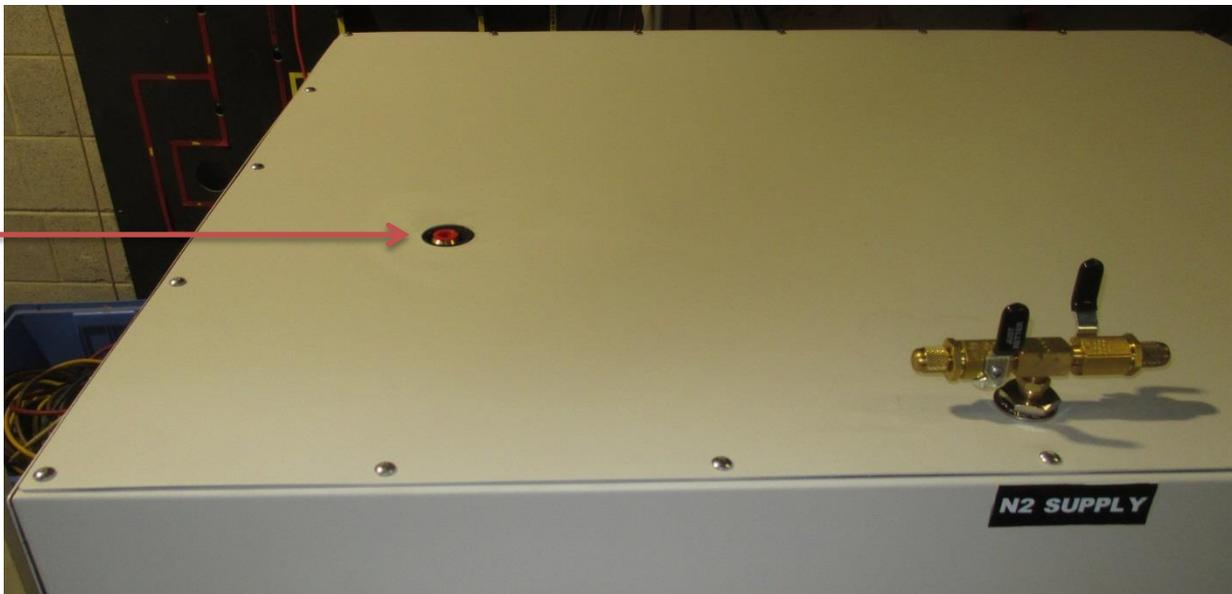
**WARNING! Do Not Plug or Restrict the Pressure Relief Valve at the top of the machine. Damage to the Machine, Property Damage and Injury May Result.**
