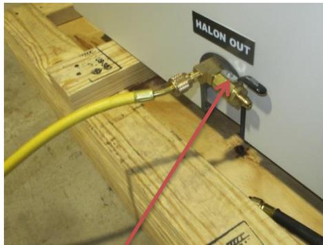
7. Open the Outlet Evacuation Valve to release the nitrogen pressure.
