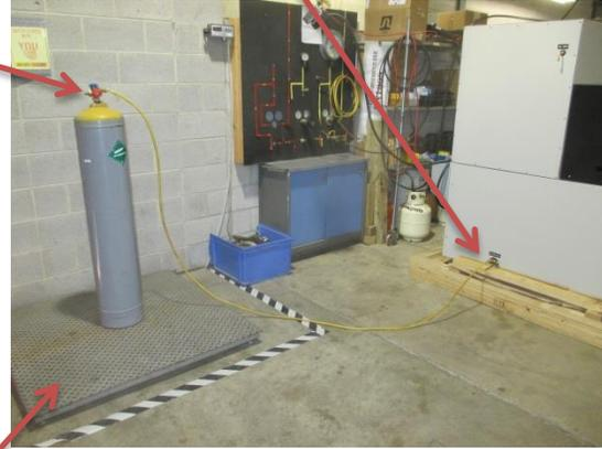
The storage container is placed on a weigh scale.
