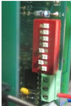
Temperature Controller Micro Switch Settings
