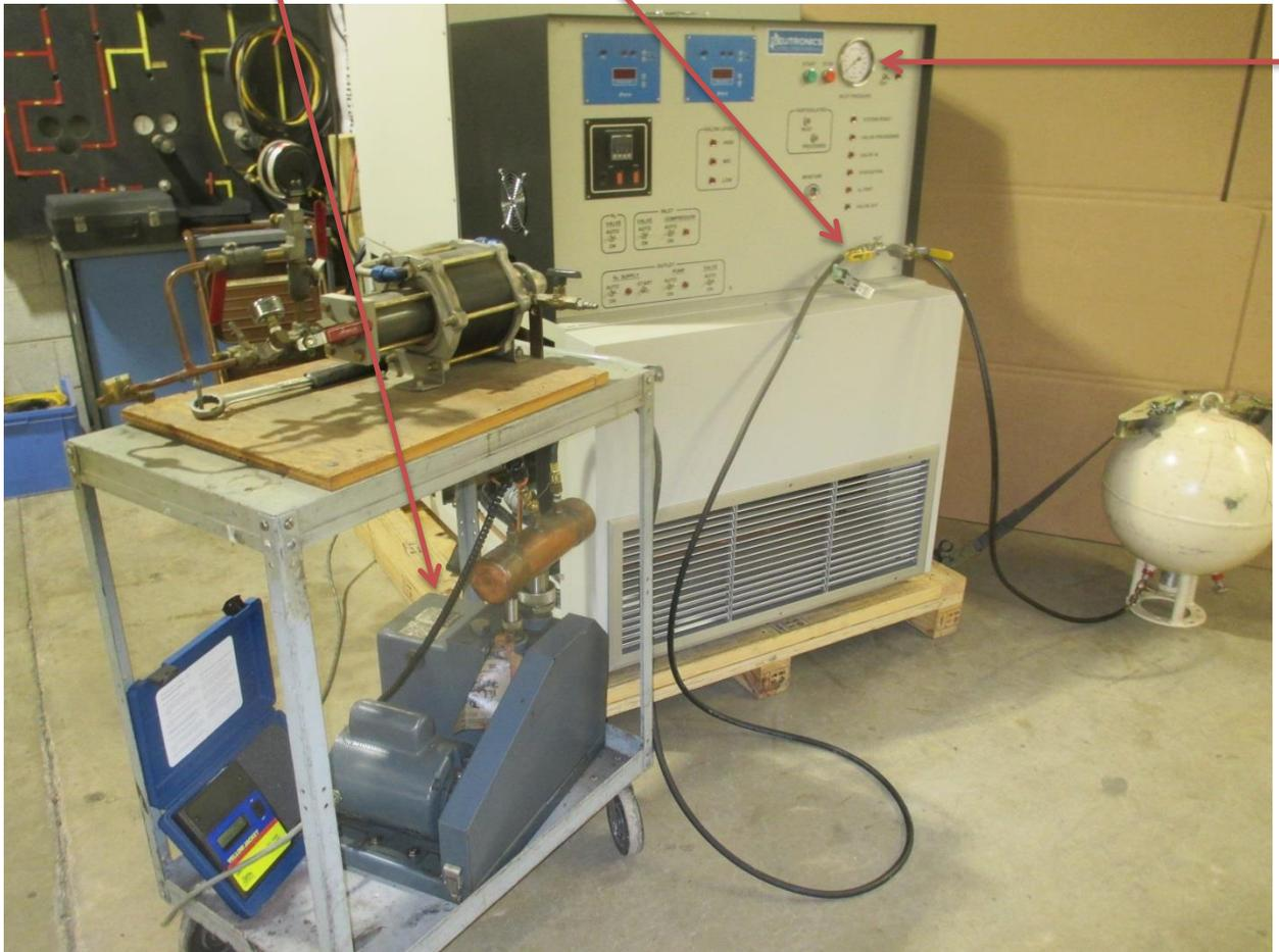
7. With the Evacuation Valve and Manual Inlet Valve still open; operate the vacuum pump to gain a vacuum indication on the Front Panel Inlet Pressure Gauge.
