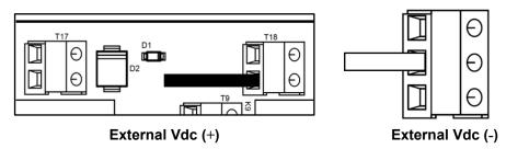
Externally derived power can also be applied to the relay output terminals to drive horns and strobes. The external source cannot exceed 30VDC. To wire external power to the relay outputs, remove the red jumper on terminal block T18 by loosening the terminal screws, wire the positive (+) of the external source to the lower terminal as shown above, and wire the negative (-) of the external source to any available terminal on the grounding terminals (terminal block T20 – T25)
