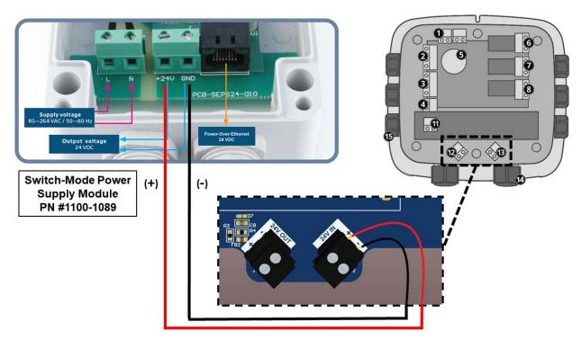
Locate the +24 VDC input terminal block (#13) and unplug it from the controller.
