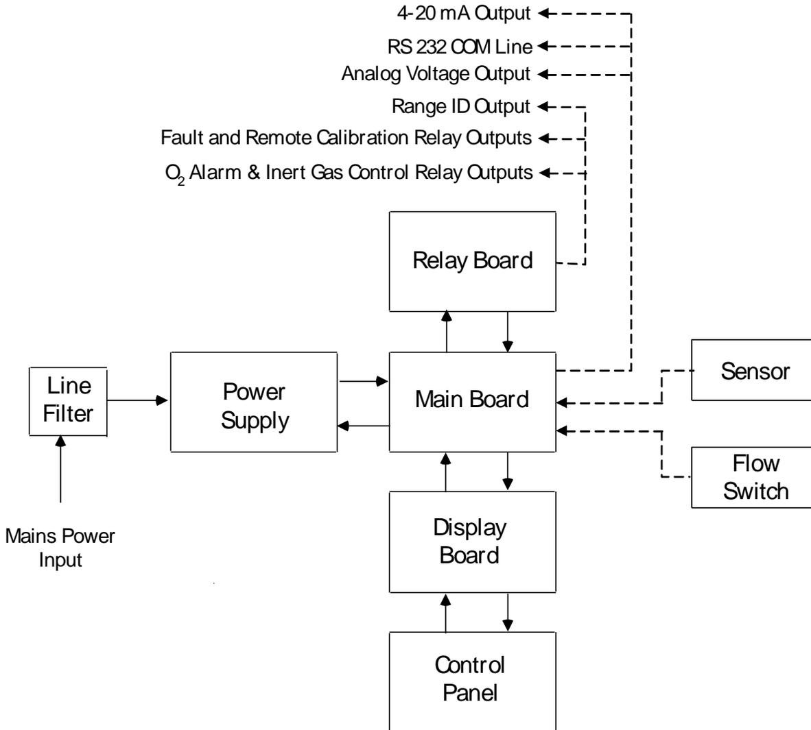
Figure 5 – Analyzer system configuration
