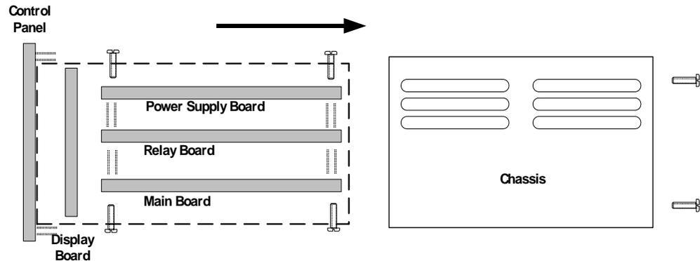
Figure 3 – Basic analyzer components
