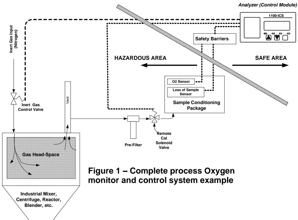
**Figure 1 – Complete process Oxygen monitor and control system example**
