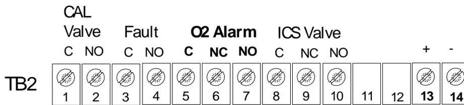
**2.1.3.4 Inert Gas Control Relay Outputs**
