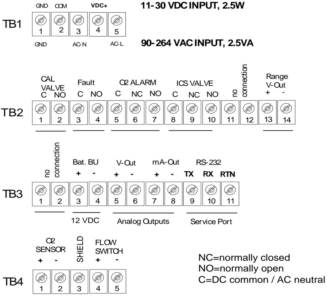
Figure 9 - analyzer electrical
