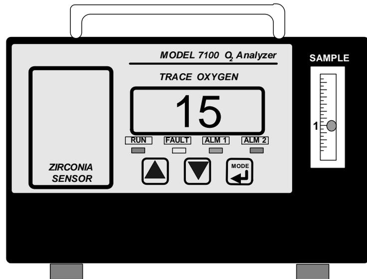
At the heart of the analyzer is a Neutronics Inc. micro-Zirconia ceramic oxygen sensor. The Zirconia sensor is a solid state device which assures reliability and fast response for critical measurements. Another advantage is since the sensor is a solid state device, it is unaffected by dry atmospheres, is undamaged by extremely cold storage temperatures (or power down situations in cold environments), and has indefinite storage life.
