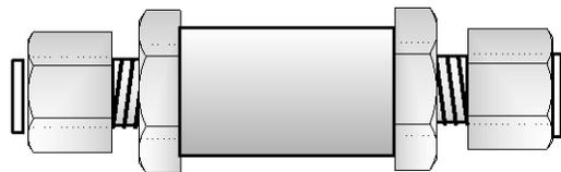
Figure 10 Bypass Valve
