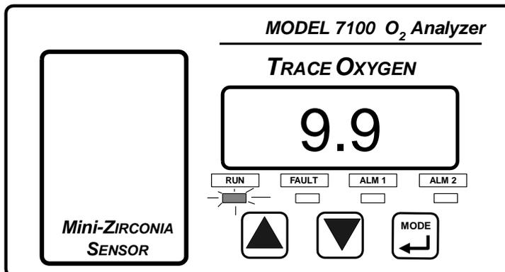
The Model 7100P Portable analyzer will resume normal RUN mode operation when the UP, DOWN, or MODE buttons have not be pressed within a 120 seconds period.
