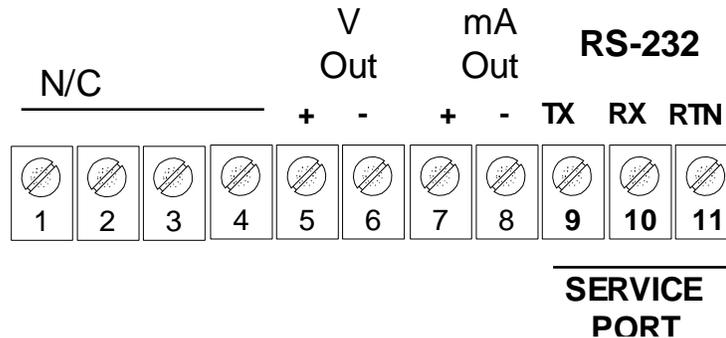
Access to the Serial Service Port may be made through a terminal emulator program such as HyperTerminal available in Windows 95/98:.
