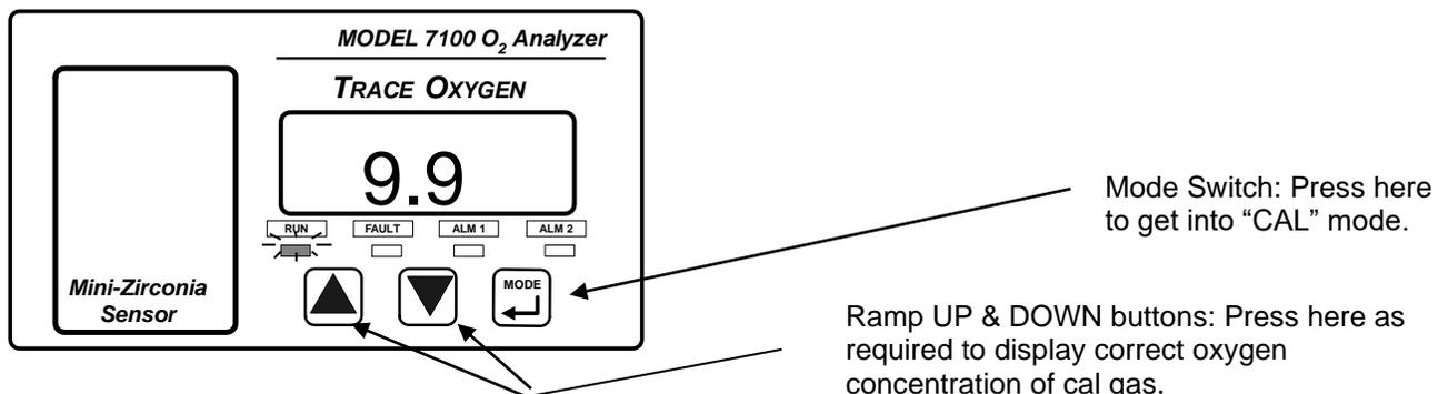
3. "CAL" will be displayed. The Green LED "RUN" will blink fast. Press the UP and Down arrows as needed to show correct PPM oxygen on the display.
