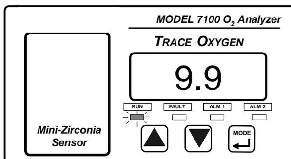
**NOTE: DO NOT CALIBRATE WITH A ZERO GAS. SETTING ZERO WILL CREATE ERROR IN THE MEASUREMENT CALCULATIONS!**
