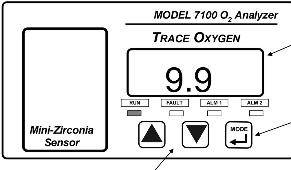
The numeric display features large, super bright LEDs. There are two modes of display: When the analyzer is in the "out of normal operating range" measurement range, the display will flash bright to dim.
