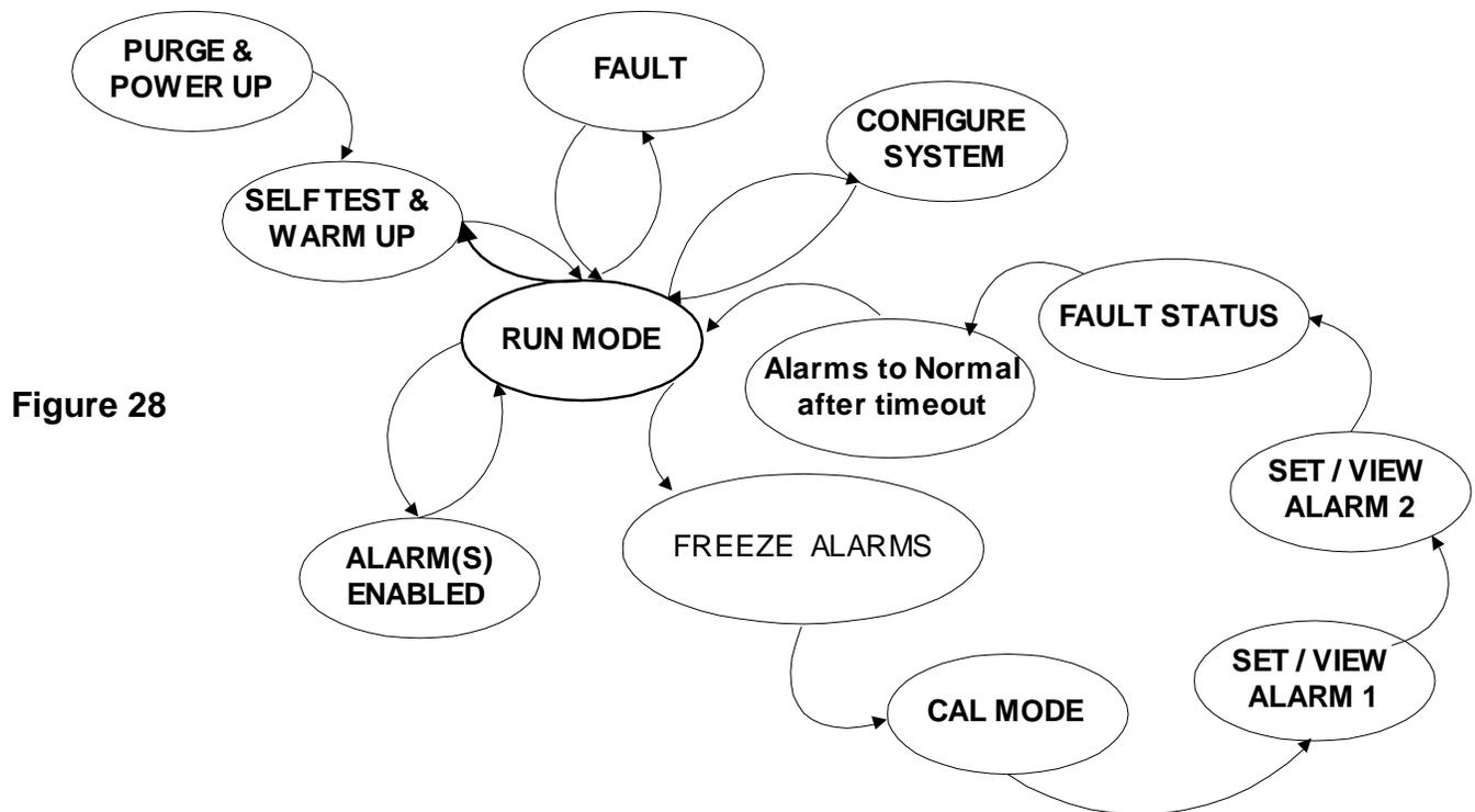
After the unit has been calibrated on a known gas source, it can be used in normal operation. There are six main modes of operation once the system has been powered up and the self test/warm up period is completed: **RUN, Calibration, Set Alarms, Alarms Active, Fault, and SELF-TEST.**
