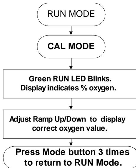
Calibration gas should be applied to the analyzer at a similar flow rate and pressure to that of the sampled gas. Be sure to allow the calibration gas to flow to the sensor until the display has stabilized. The stabilization period allows time for the calibration gas to flush the gas in the sampling lines.
