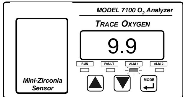
*Ascending or Descending Trip?* Alarms may be configured with ascending or descending trip. An ascending trip means the alarm will activate due to an increase in oxygen concentration above the setpoint programmed into the Model 7100. Descending trip will cause an alarm to activate due to a decrease in oxygen concentration below the setpoint programmed into the Model 7100. The oxygen concentration setpoints are programmed as described below.
