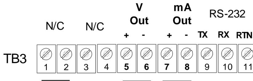
Two wires are required for each output. Individually shielded twisted pairs using stranded wire conductors are suitable for the connections. The shield should be drained to dc ground at the auxiliary equipment.
