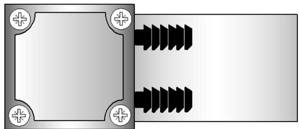
**1.3.10 Bypass Valve:** The Bypass valve creates a constant backpressure ( 5 psig) on the sensor orifice and hence a stable sensor flow. Additionally, the Bypass valve ensures a fast response time by allowing a portion to bypass the sensor and continuously sweep the system of previous gas samples.
