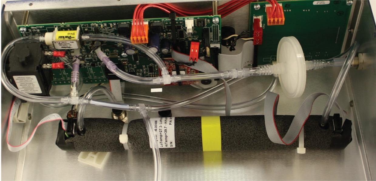
**Figure 2. Internal Components Showing the IR Sensor (Bench) of a PGM-IR**
