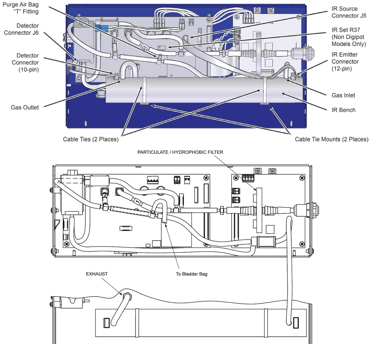
**Figure 5. Monitor Components in Various PGM-IR Models**
