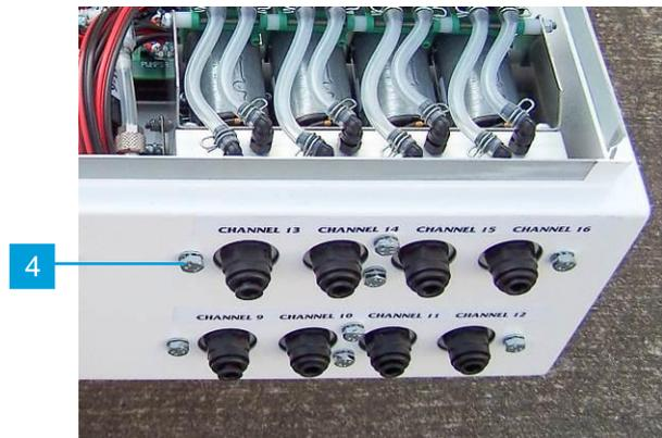
To install the new SAMM block, fit the new SAMM block in the vacant position. (Note: It will only fit with the 8 short sampling pipes facing towards the front of the enclosure.) Fit the shake-proof washers and fixing screws and tighten. Re-attach the hose to the non-return valve of the new SAMM block and plug in the SAMM block wiring connector.
