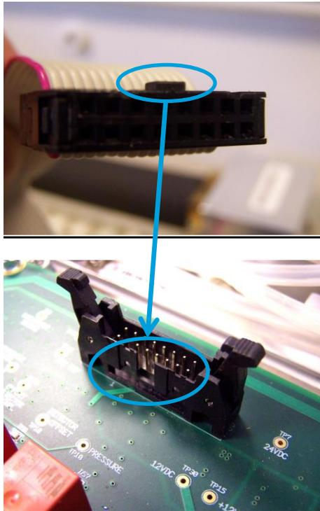
NB: If the ribbon cable is installed incorrectly, the monitor will not power up although some LEDs may light up. In this instance, correct the connector orientation and the monitor should power up properly.
