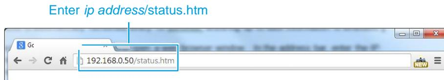
The following screen will be displayed. This page shows the current status of all channels currently being monitored by the 3300RM2. If a channel has encountered an alert, alarm or critical event, it will be highlighted using the relevant colour.
