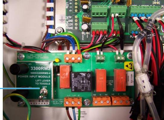
Disconnect the SAMM module wiring from the network module by unclipping the relevant connector **(2)**.
