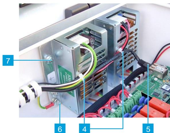
Secure the new power supply in place with fixing nuts **(7)**, including new shake-proof washers. Connect the new cables **(2)(3)** and route through the cable trunking. Check all connections are secure. Switch the main isolator **(1)** to the 'On' position. Close the enclosure door and secure with locking bolts. Reinstall the mains supply.
