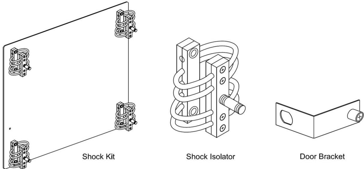
Push the monitor onto the four mounting pins of the shock isolators and secure in place using the fixings supplied with the mounting kit.
