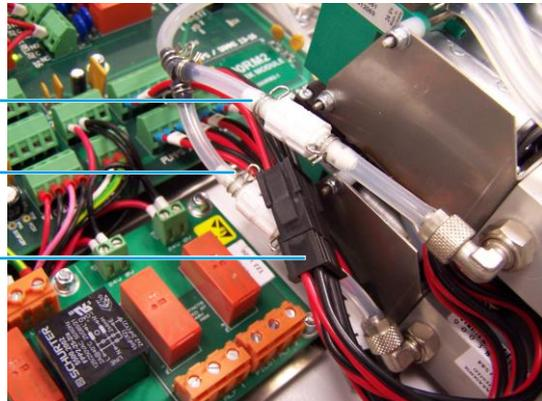
Remove the four fixing screws **(4)** that are holding the SAMM module to the base of the enclosure, being careful not to damage the gasket between the SAMM and the inside of the enclosure.
