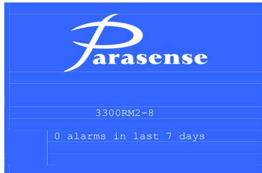
The home screen is shown when the system is first accessed, or if no buttons have been pressed for 3 minutes. The home screen displays the product name and number of working SAMMs. Also displayed is the number of alarms (maximum of 100) that have occurred over the recording period (1 to 14 days as set during configuration). Pressing the  button on the keypad accesses a primary selection menu:
