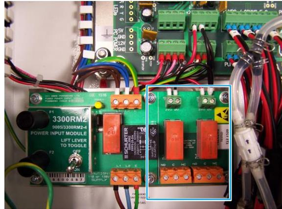
Pilot Relays on Power Input Module
