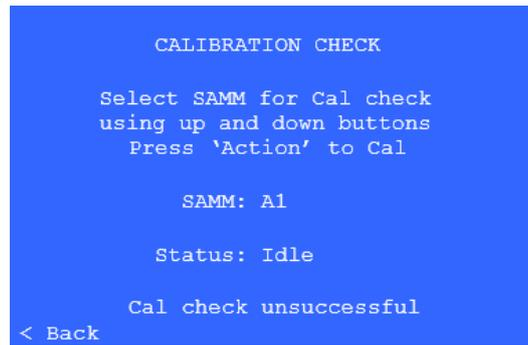
When the calibration check has completed successfully, pressing the <Back button will take you to the SAMP Test screen, where you must perform a SAMP Test to verify the correct operation of the monitor, alarm relays, associated field wiring and annunciators. If unsuccessful, see below for further instructions.
