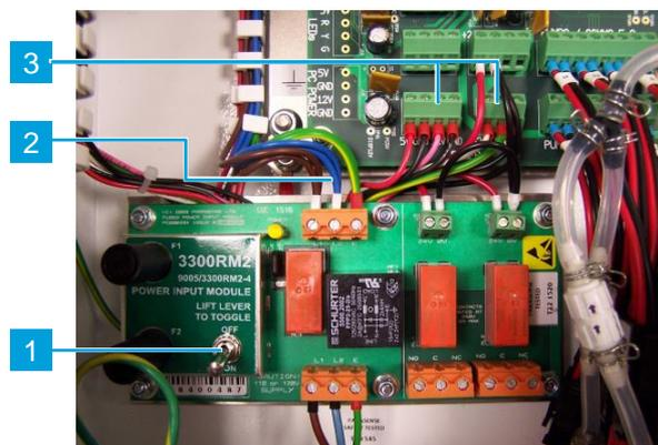
*Noting the sequence* - Disconnect the mains supply cables to the power supply **(2)** and release them from the cable trunking. Disconnect the output cables from the power supply **(3)** and remove them from the cable trunking. Unplug the CAT5 connector **(5)** adjacent to the PSU. Disconnect the Earth strap **(6)**. Unscrew the four fixing nuts **(7)** that hold the power supply in place. Remove the power supply and cables.
