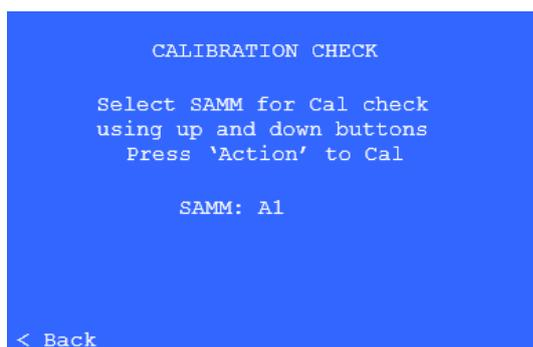
The SAMP will reflect A1 or L1 as configured. Calibration Check is performed using SAMP #1.
