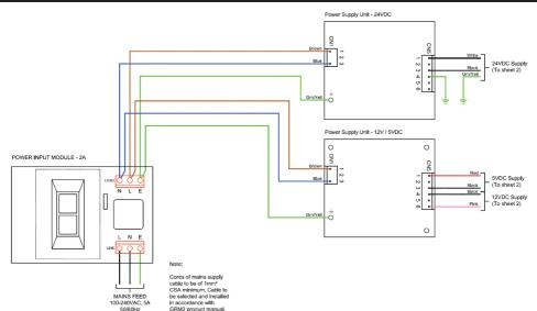
Each monitor requires an Earthed, AC single phase mains supply in the range 100 to 240 volts, 50 to 60 Hz, protected by a 5 amp fuse or similar over current circuit breaker. Power consumption for a GRM2 Monitor is 65 watts.
