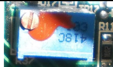
Figure 4: R37 Component (On Non Digipot Models Only)
