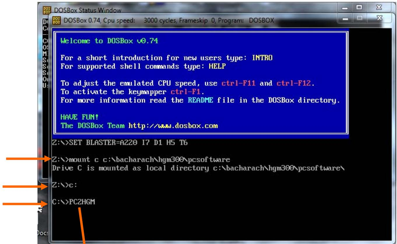
6. PC software will be launched and setup data collected from the monitor.
