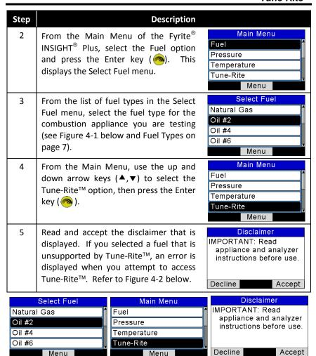
Figure 4-1. Fuel Selection Screens for Supported Fuel
