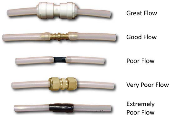
Figure 4. Tubing Connections (Best through Worst)
