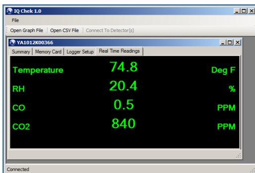
**Figure 3-3. The Real Time Readings Tab**
