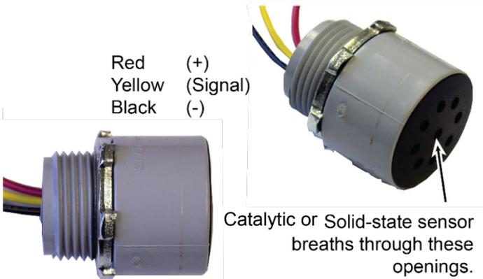
Figure 3-2. Remote Sensor Housing
