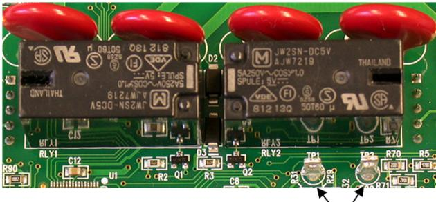
**Figure 4-3. Locations of Test Points TP1 and TP2**
