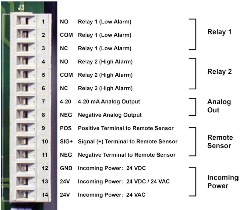
Figure 3-3. Wiring Connections for GDC-350 Types A, B, and D
