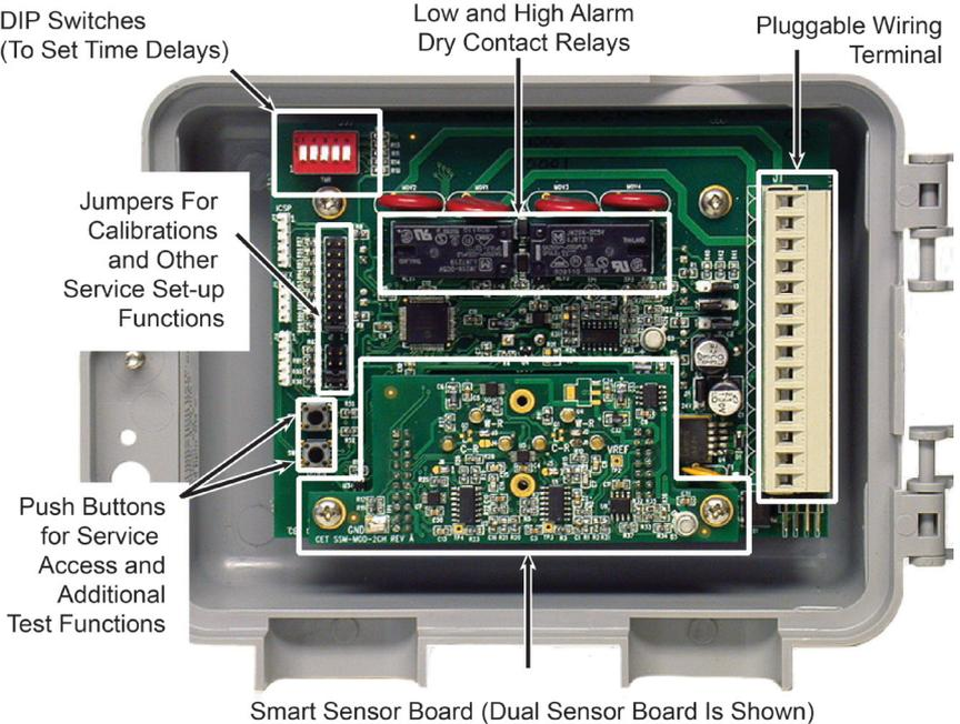
**Figure 1-3. Interior Components of the GDC-350**
