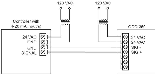
**Figure 3-5. Proper Wiring Examples**
