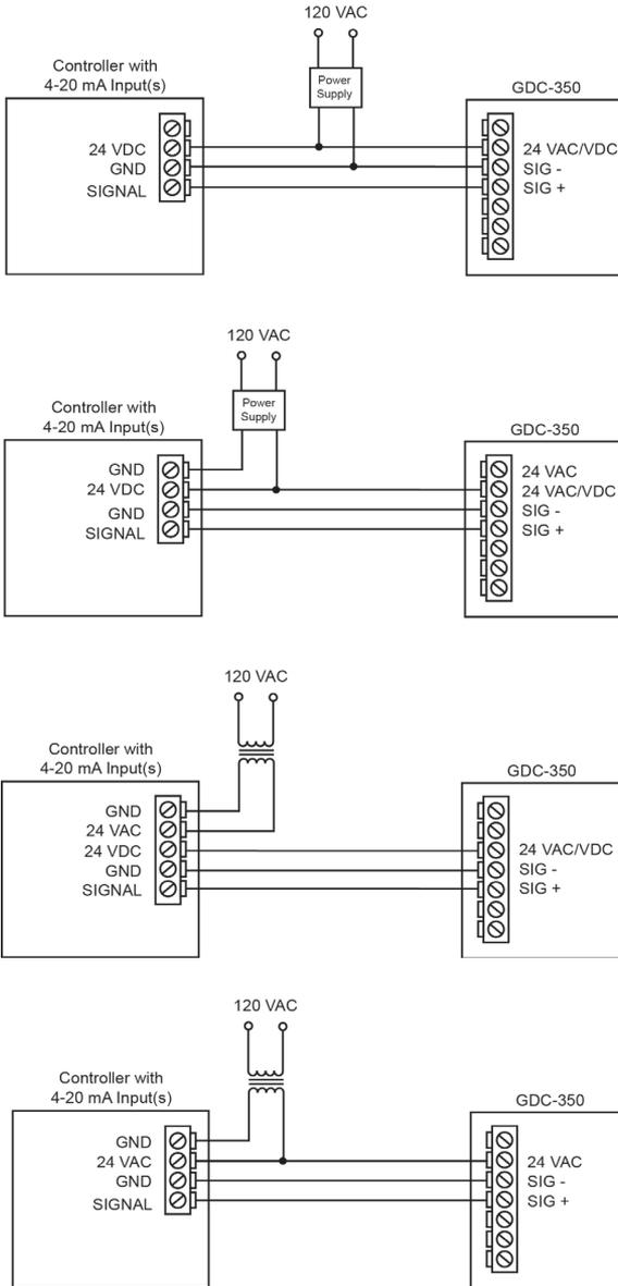
**Figure 3-5. Proper Wiring Examples (Continued)**
