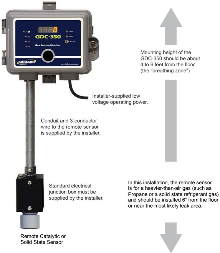
**Figure 3-8. Sample Type “B” Installation**
