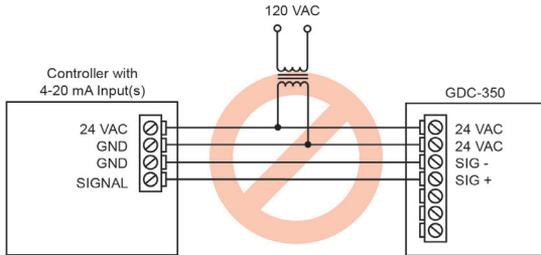
**Figure 3-6. Improper Wiring Example**
