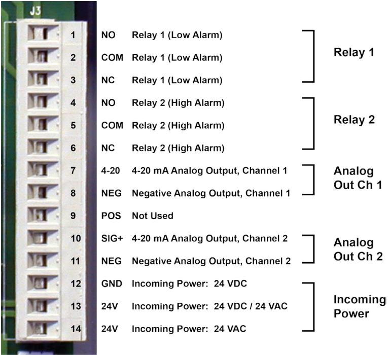
**Figure 3-4. Wiring Connections for GDC-350 Type E**
