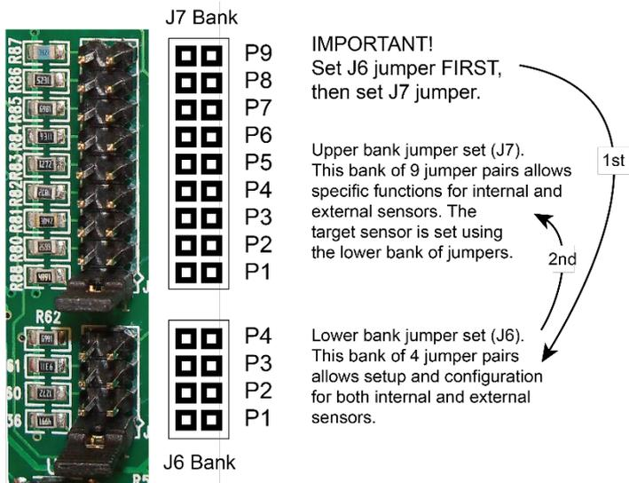
**Figure 4-2. J7 (Top) and J6 (Bottom) Jumper Banks**
