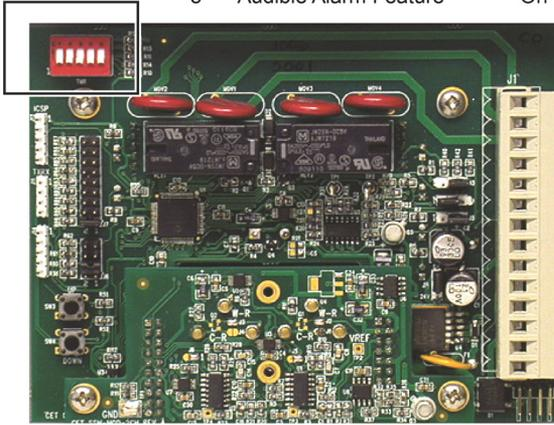
Figure 4-1. DIP Switch Settings for Alarms
