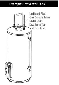
Domestic hot water tanks with the 'bell' shaped draft diverter can be accurately tested by inserting the probe tip directly into the top of the fire tube below the diverter.
