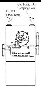
Condensing furnaces/boilers can be tested through a hole drilled in the plastic vent pipe (when allowed by the manufacturer or local authority of jurisdiction) or taken from the exhaust termination.
