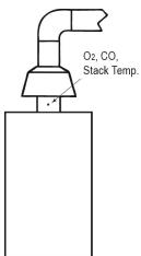
Boilers, which have a 'bell' shaped draft diverter on top, should be tested directly below the diverter through a hole drilled in the vent connector.
