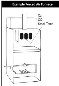
For atmospheric burner or gravity vented, forced air heating equipment with a clamshell or sectional heat exchanger design, test each of the exhaust ports at the top of the heat exchanger. The probe should be inserted back into each of the exhaust ports to obtain a flue gas sample, before any dilution air is mixed in.
