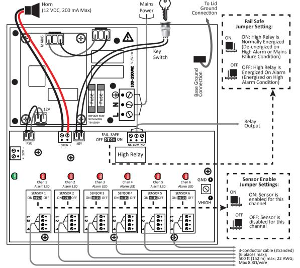
Ensure that connections 1 to 4 on each sensor connect to their corresponding numbers on the terminal block in the main alarm unit, otherwise the system will not function correctly and could be
