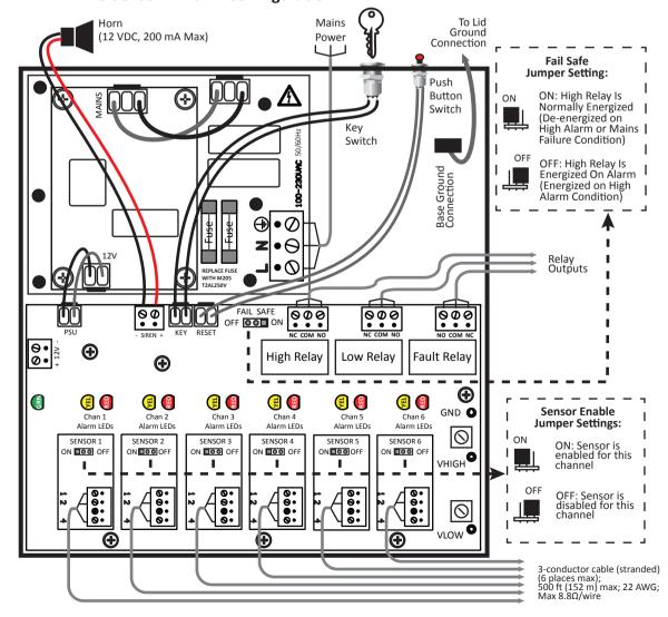
Ensure that connections 1 to 4 on each sensor connect to their corresponding numbers on the terminal block in the main alarm unit, otherwise the system will not function correctly and could be damaged
