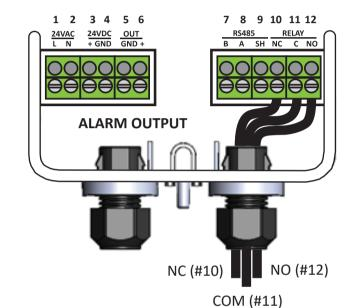
NOTE: After wiring is completed, carefully re-assemble the enclosure. After installation is complete, be sure to refer to the User Manual (part number 6490-9000) at www.MvBacharac-
