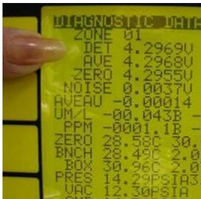
Figure 7. Detector voltage should be between 4.2 and 4.3 VDC
