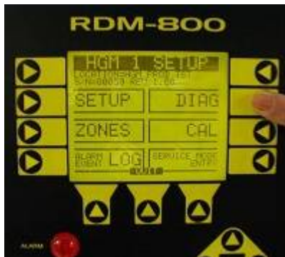
Figure 6. Push DIAG button to display DIAGNOSTIC Screen
