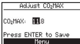
5. Save the selection and return to the Combustion Test HOLD screen or **ESC** to cancel and return to the select Fuel Menu. From the Fuel Menu, press **ESC** again to return to the Main Menu.
