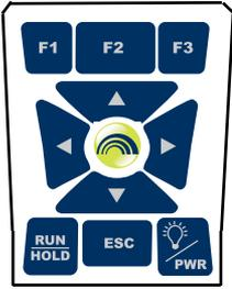
Note that a push button may perform several functions, depending on the analyzer's model number and the screen that is displayed.
