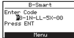
3. Use the ▲▼ buttons to enter the 10 digit alphanumeric code supplied with the B-Smart sensor. Use the ◀▶ buttons to move the cursor across the screen. Press **ENTER**.
