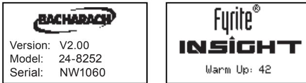
4. After the 60 second warm-up period is completed, the instrument will display the Combustion Test HOLD screen.
