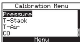
7. Use the **▲▼** buttons to select the desired sensor channel to be calibrated, and then perform the calibration procedure for that sensor as described in the following sections.
