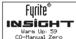
**Auto Zero:** When the CO channel is set to auto zero, the CO sensor is zeroed to the ambient CO level during start up.
