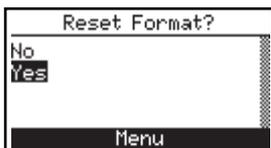
4. Select **Yes**. Press the **ENTER** button to reset the format and return to the Run/Hold format options.
