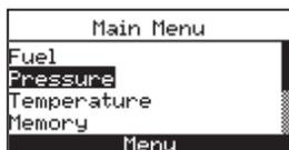
4. Before taking a measurement, the pressure sensor may need to be re-zeroed if it is not already displaying zero with both pressure ports open to the atmosphere. If necessary, zero the pressure sensor as follows:
