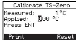
*“Measured” is the current temperature reading, while “Applied” is a known temperature that will be applied for calibration purposes.*
