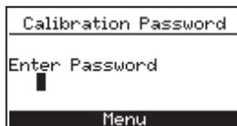
5. Before calibration can begin a 4-place numeric password must be entered. Use the **▲▼** and **◀▶** buttons to enter the password. (Note that the default password is 1111)
