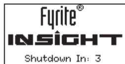
If the analyzer was not purged with fresh air then the analyzer may remain ON with its pump running and display the message “PURGING SENSORS” as the result of combustion gases still being present inside the analyzer. At this time the operator should ensure that the probe is removed from the stack, allowing the analyzer to purge itself with fresh air. The 5-second-shutdown sequence will not begin until the gas levels inside the analyzer drop below predetermined levels.
