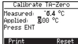
*“Measured” is the current temperature reading, while “Applied” is a known temperature that will be applied for calibration purposes.*
