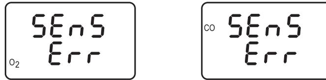
An O<sub>2</sub> sensor error is displayed if the analyzer determines during the warm-up cycle that the oxygen sensor's output is too low for it to be usable. However, in the extreme condition when the O<sub>2</sub> sensor has *no output*, a sensor error will not occur. Instead, the O<sub>2</sub> reading will be 0.0 as displayed in the O<sub>2</sub> Screen or the CO & O<sub>2</sub> Screen.
