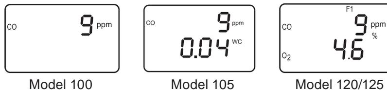
3. Insert the analyzer's probe into the area to be tested and observe the detected CO level on the LCD.
