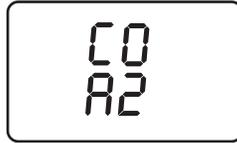
1. Enter the Setup Mode per Section 3.5.1. If necessary, repeatedly press the **ENTER** button until “CO” is displayed.
