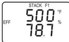
The STACK reading is the temperature measured at the tip of the probe.
