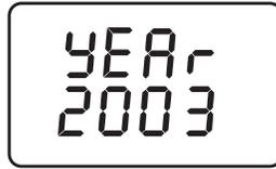
1. Enter the Setup Mode per Section 3.5.1. If necessary, repeatedly press **ENTER** until the Year Setup Screen is displayed.
