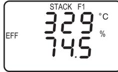
2. Position the probe in the flue-gas stream to obtain the hottest “Stack” reading. *Locating the highest stack temperature is very important for accurate efficiency calculations.*
