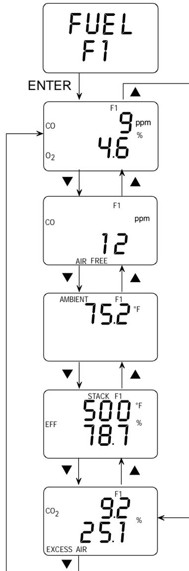
**Figure 4-2D. Model 120 Run Mode Screens**
