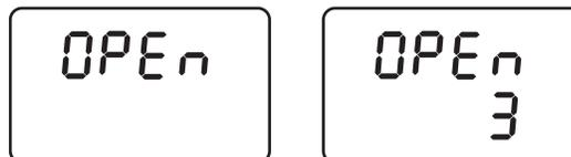
3. Press the ▲ or ▼ button to scroll to the desired memory location, and then press **ENTER** to recall the stored data and return to the Hold Mode. While in the Hold Mode, the recalled data can be viewed using the ▲ and ▼ buttons, or printed per Section 4.9.
