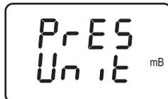
1. Enter the Setup Mode per Section 3.5.1. If necessary, repeatedly press the **ENTER** button until “PrES” is displayed.
