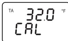
3. Set the simulator to 32.0 °F (0 °C); then use the ▲ and ▼ buttons to set the displayed value to match the simulator's value.
