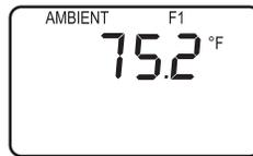
The AMBIENT reading is the combustion-air temperature in either °F or °C that is used for efficiency calculations. This temperature is measured by either the T-AIR thermocouple on a continuous basis (Model 125), or by the T-STACK thermocouple during start-up (Model 110/120/125). If *neither* thermocouple is installed when the analyzer is turned ON, then this temperature reading comes from a temperature sensor located inside the analyzer. Refer to Section 4.2.1.
