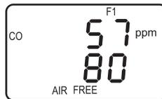
The CO AIR FREE reading is a calculation of the exact ppm concentration of carbon monoxide at the flame if oxygen were 0.0% in accordance with ANSI standard Z21.1.
