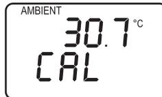
2. Use the ▲ and ▼ buttons to set the displayed value to match the reading of a calibrated thermometer at room temperature.
