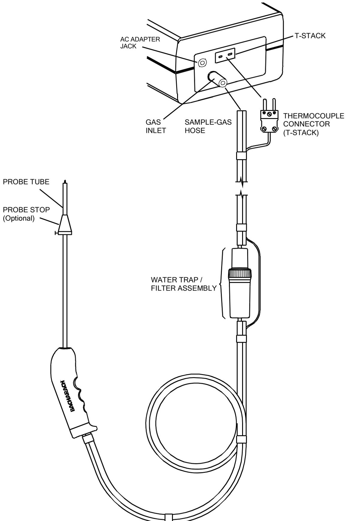
**Figure 3-2C. Connecting the 0019-7111 Probe (Model 110/120)**
