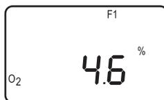
The O<sub>2</sub> Screen shows the measured percentage of oxygen present in the flue-gas stream.
