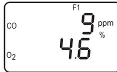
The CO reading is a measurement of how much carbon monoxide in ppm is present in the flue-gas stream. Note, however, that the amount of CO displayed may be diluted by secondary air (refer to Section 4.13.12 CO Air Free Screen).
