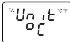
1. Enter the Setup Mode per Section 3.5.1. If necessary, repeatedly press the **ENTER** button until “Unit” is displayed.
