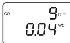
3. The draft reading should be zero when sampling room air. If not, press the ▼ button *once* to display the Draft Zero Screen, and then press the **ENTER** button to zero the draft channel to ambient atmospheric conditions.
