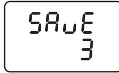
3. Press **ENTER** to save the test data and return to the Hold Mode, or press **HOLD** to return to the Hold Mode without saving.
