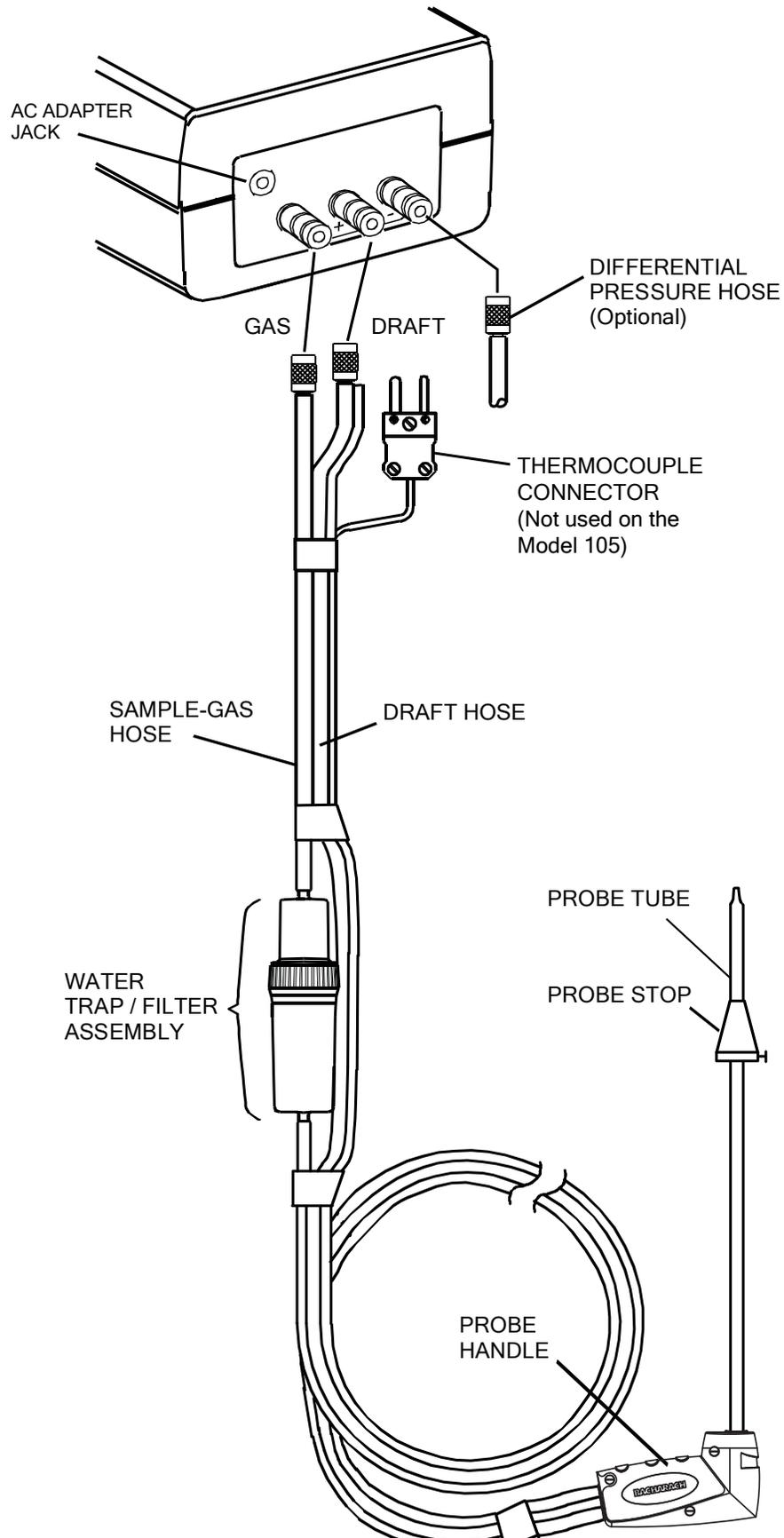
**Figure 3-2B. Connecting the 0024-3004 Probe (Model 105)**
