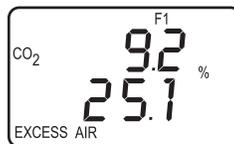
The CO<sub>2</sub> reading is a calculation of the percentage of carbon dioxide that is being produced by the combustion process.
