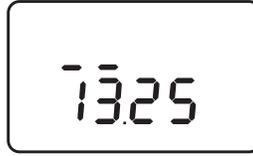
1. Enter the Setup Mode per Section 3.5.1. If necessary, repeatedly press **ENTER** until the first Time Setup Screen is displayed—the one with two bars over the hour digits.
