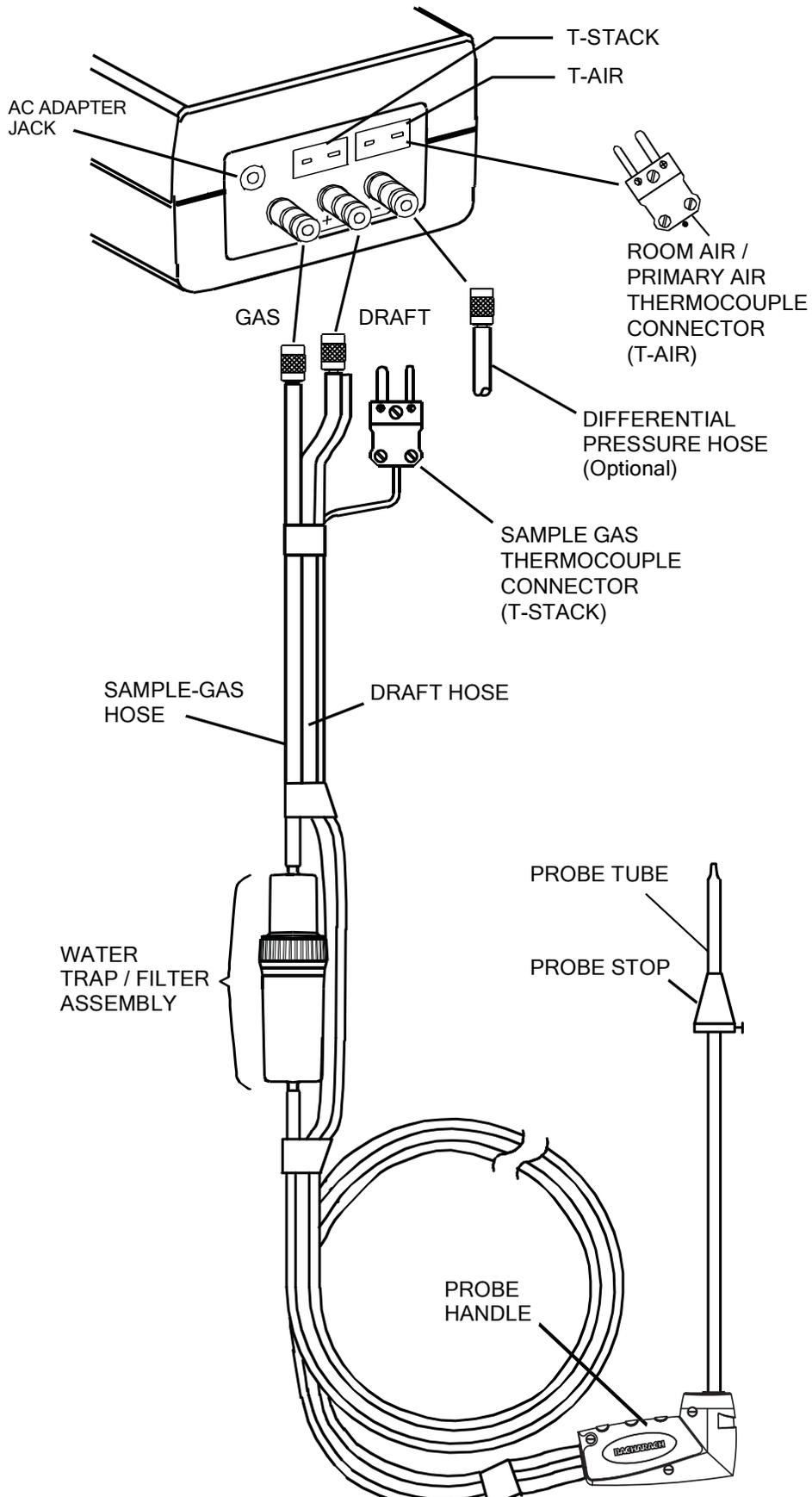
Figure 3-2D. Connecting the 0024-3004 Probe (Model 125)
