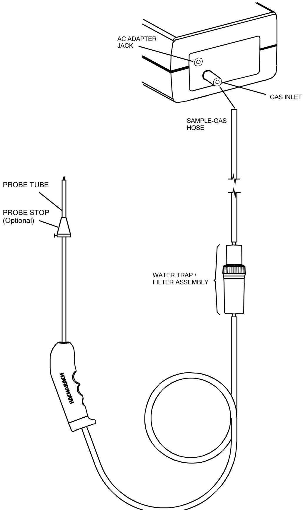
**Figure 3-2A. Connecting the 0019-7110 Probe (Model 100)**
