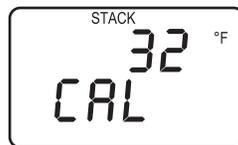
3. Set the simulator to 32 °F (0 °C); then use the ▲ and ▼ buttons to set the displayed value to match the simulator's value.
