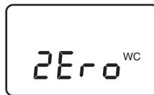
The Draft Zero Screen allows the user to manually zero the draft channel when the pressure reading is anything other than zero when measuring ambient room pressure. To zero the draft channel, remove all tubing from the analyzer's "+" and "-" ports and press the **ENTER** button.
