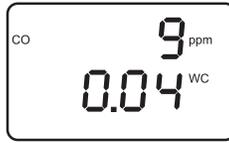
The CO reading is a measurement of how much carbon monoxide in ppm is present in the flue-gas stream. Note, however, that the amount of CO displayed may be diluted by secondary air (refer to Section 4.13.12 CO Air Free Screen).
