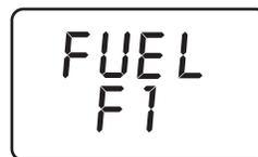
2. Press the **ENTER** button to select the displayed fuel code and enter the Run Mode.
