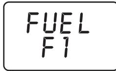
The Fuel Screen is displayed after warm-up, and is where an operator chooses which fuel is to be used by the analyzer to calculate combustion efficiency. Pressing the ▲ or ▼ button scrolls the display through the fuel codes. Pressing **ENTER** selects the displayed fuel and places the analyzer into its Run Mode. Note that the fuel code will be displayed in the top right corner of all screens while in the Run Mode.
