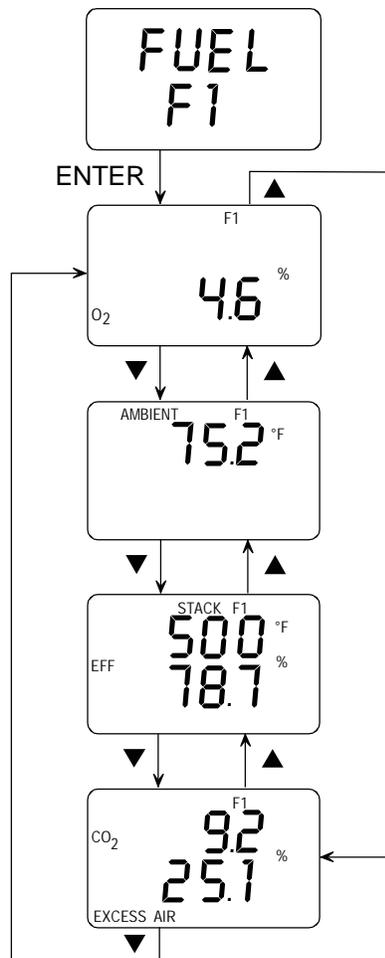
**Figure 4-2C. Model 110 Run Mode Screens**
