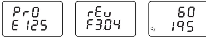
These screens show the analyzer's model number, the unit's software revision, and finally the remaining warm-up time. If an O<sub>2</sub> sensor is installed, then its current output level is also displayed.
