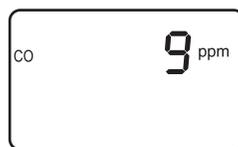
The CO Screen is displayed after warm-up and shows the current CO level in ppm. If the probe is being used, insert the probe tip into the area to be sampled.
