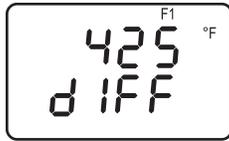
The Temperature Differential reading is the measured difference between the temperatures being measured by the T-STACK and T-AIR thermocouples.
