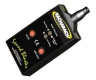
Some Tru Pointe<sup>®</sup> Ultra HD kits include Bacharach's ultrasonic sound generator, the SoundBlaster<sup>®</sup>. The SoundBlaster<sup>®</sup> is used to artificially pressurize items and detect potential leaks using a 115dB ultrasonic tone. The Tru Pointe<sup>®</sup> Ultra HD can detect the tone as it escapes in areas that are not under pressure.
