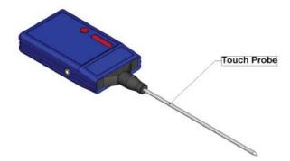
The patented Touch Probe accessory is a device that converts solid-borne sounds into airborne sound the Tru Pointe<sup>®</sup> Ultra HD can detect. For example, the sound of an internal leak in a water valve will travel to its surface. Touching the surface of the valve with the Touch Probe transfers the ultrasound into the probe and converts it to airborne ultrasound. To install the Touch Probe:
