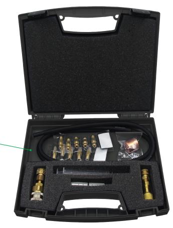
The kit comes complete with High Side couplers for both R-12 and R-134a systems, 10 disposable cartridges, a flow meter, syringe, and hose, housed in a storage case.
