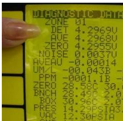
Figure 7. Detector voltage should be between 4.2 and 4.3 VDC
