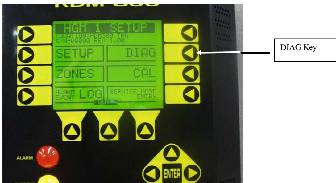
2. Record the following values from the DIAG Screen: DET, AVE, ZERO, NOISE, PPM, ZERO, BENCH, BOX, PRES, VAC and AMB. **Verify that the VAC reading is less than 12.5 PSIA.** If it is not, please contact Bacharach at [help@bacharach-inc.com](mailto:help@bacharach-inc.com) or call 800-850-0044 for assistance.
